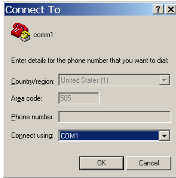
Figure 11-2: Connecting to the Computer's Serial Port
