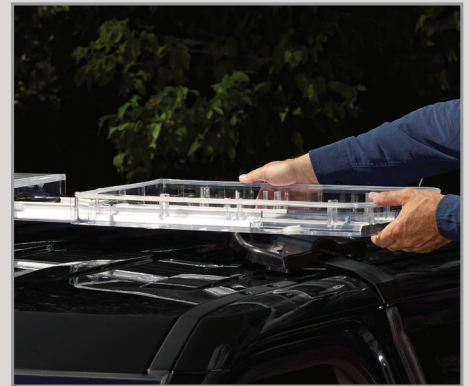
3 The base slides off for quick replacement.
